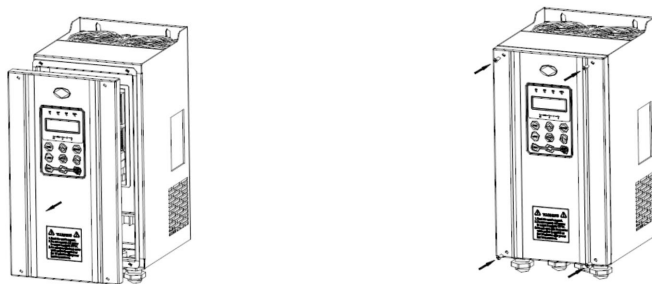
Figure 3- 11 Cover installation of IP54 level AC drive
